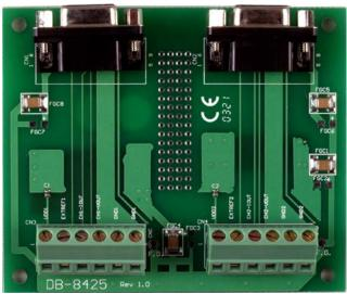
Two Female DB9 to Screw Terminal Board for PISO-DA2U
